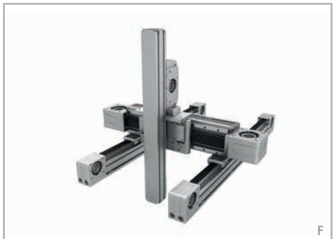
F - Linear units: X Axis 2 E-SMART - Y Axis 1 R-SMART - Z Axis 1 S-SMART Connection kit: 2 fixing brackets Kit for 2 R-SMART (Y axis) on 2 E-SMART (X axis). Connection plate Kit for S-SMART (Z axis) on 2 R-SMART (Y axis). Parallel Kit
